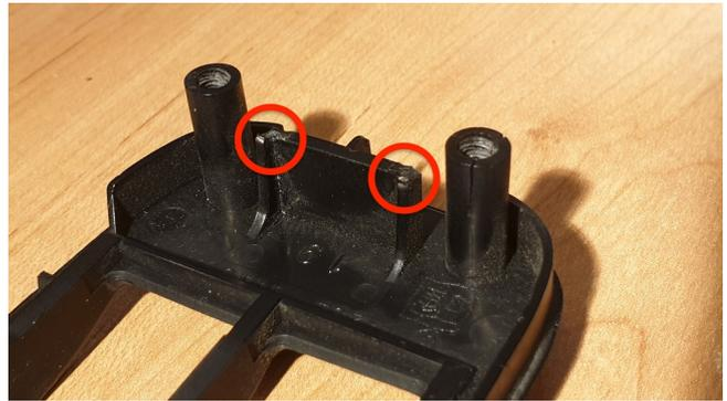
5. Fit the WinFix in place of the broken clip.
